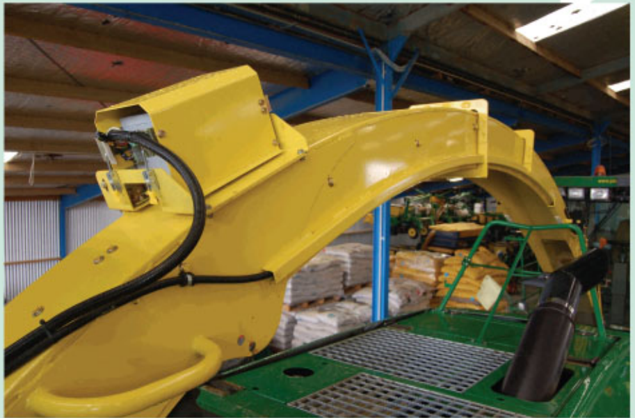
This photo shows an NIR mounted on the spout of the forage harvester. The NIR is responsible for measuring the forage dry matter percentage.
